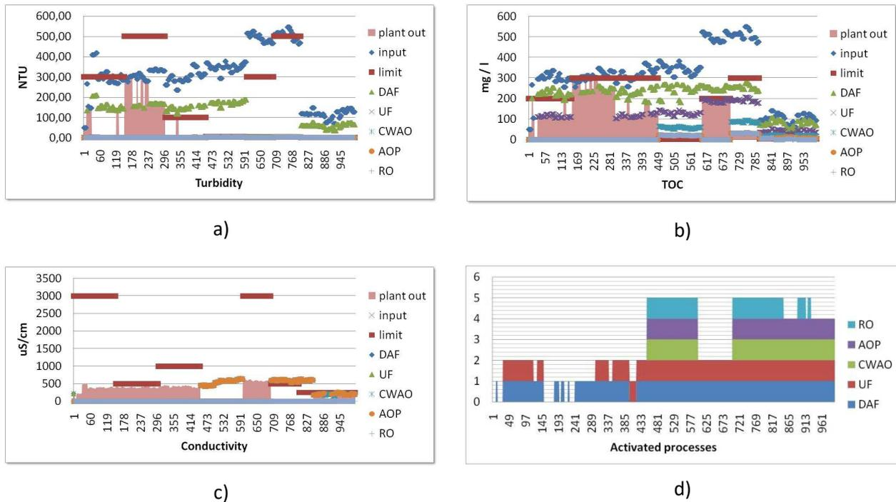
**Figure 3a) (top left hand side) Simulated turbidity effluent values of each process evolution along time; 3b) (top right hand side) Simulated TOC effluent values of each process evolution along time; 3c) (bottom right hand side) Conductivity effluent values of each process evolution along time; 3d) (bottom right hand side) Active processes evolution along time**
