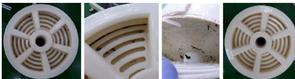
Figure 4 Autopsied membranes: external inspection
